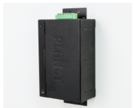
Side Wall Mounting (Space saving)
